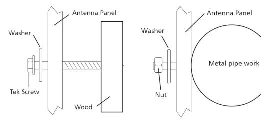
4. Using the defined mounting holes, mount the Antenna Panel on the outside of the animal handler so that the middle of the Antenna Panel matches the average height.
